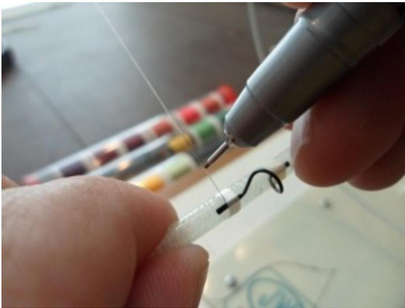
The wrap is backed off the blank and the space in between the two dots is “colored in”.
