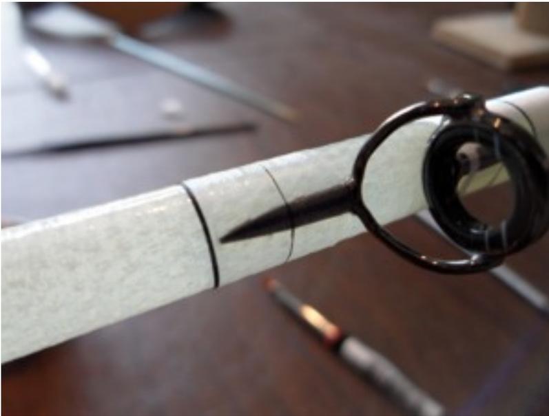
As you can see (sorry the picture is a little fuzzy on this one) on this foot a bubble formed on the side of the guide foot.
