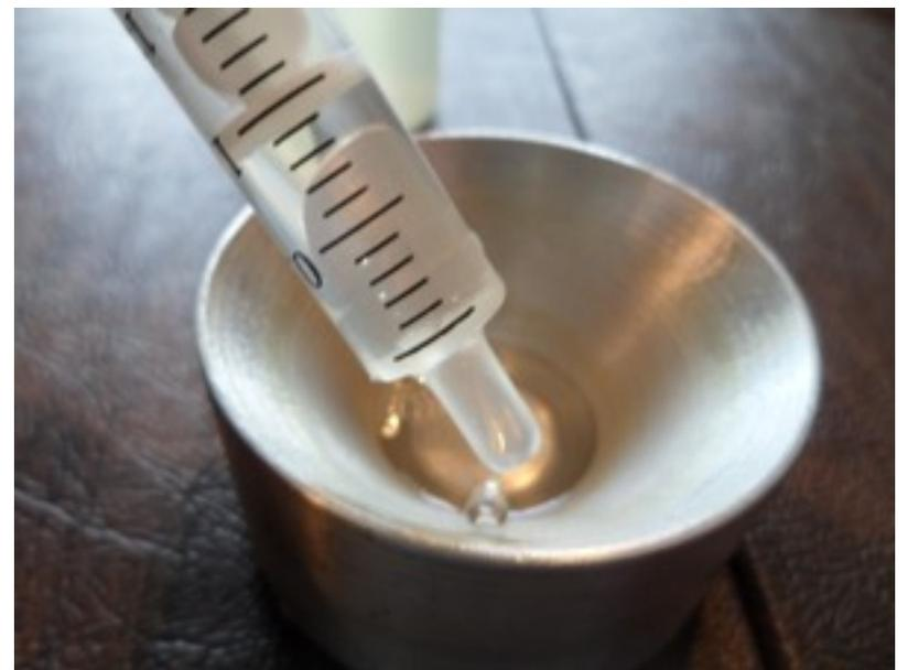
resin, 1 part hardener, and 1 part acetone. (All by volume) The acetone thins the mix and allows for quick and thorough penetration of the wraps. This is critical for the first stage as you want to eliminate any chance of getting bubbles, or micro bubbles, in the finished wrap.
