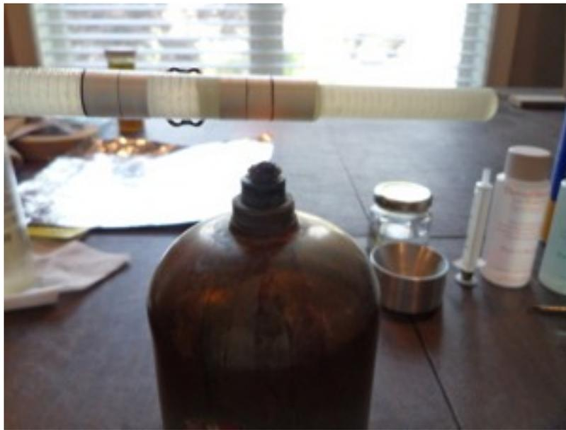
To begin the wraps are passed over an alcohol torch to singe away any "fuzzies" in the silk. Denatured alcohol burns at somewhat low temperatures which allows the wrap to be rotated quickly in the flame without scorching. You'll notice in the pictures that the torch doesn't even appear to be lit. The flame is "blue" and doesn't show in the pictures.
