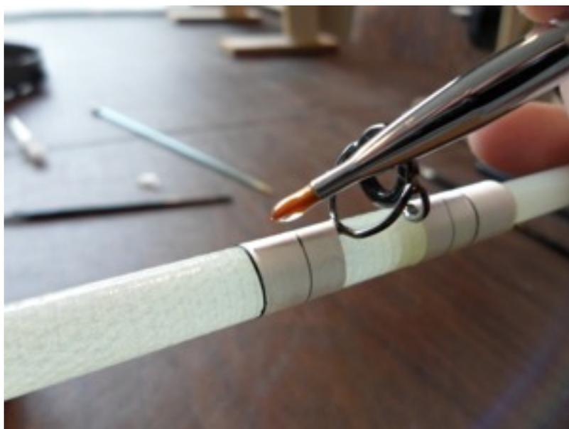
Now the finishing of the wrap begins. A large drop of epoxy is placed on top of the guide foot and then worked around the wrap, thoroughly coating everything but done with care so as not to spill onto the blank at this point.
