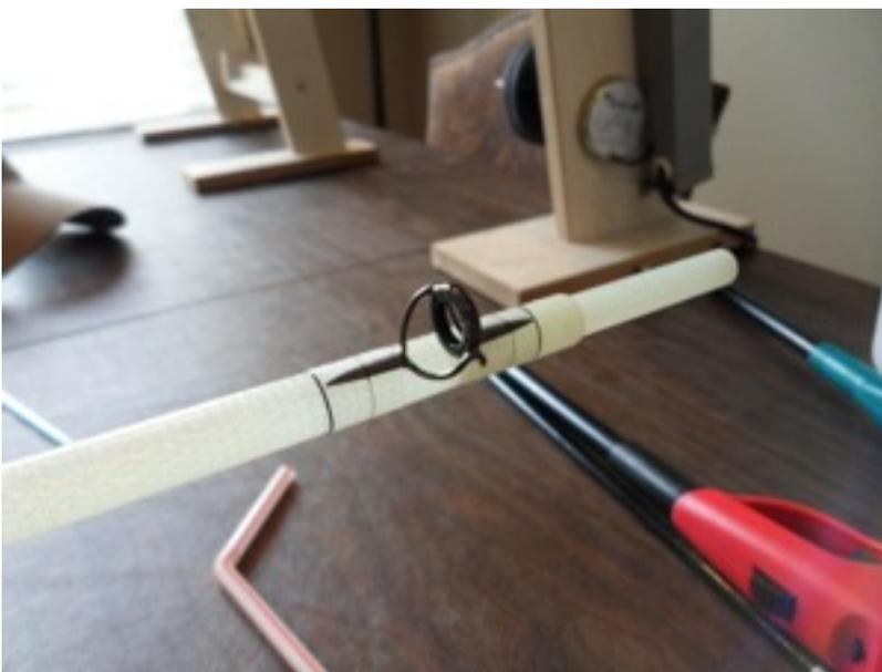
At this point as much epoxy as possible is wicked away leaving the wraps just appearing damp.
