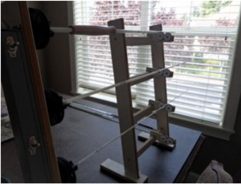
The balance of the wraps and trim bands are completed in the same manner and the rod is placed in the dryer.
