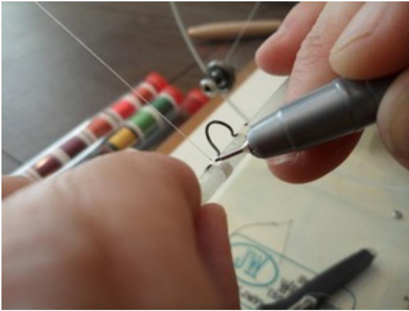
The dot is allowed to dry for a moment and a turn of thread is made and another dot of ink is carefully placed to meet the first at the end of the wrap. Care needs to be taken and you can work your way slowly toward the exact point where the beginning and end of the wrap meet. (This is where the optivisor or reading glasses come in handy.)
